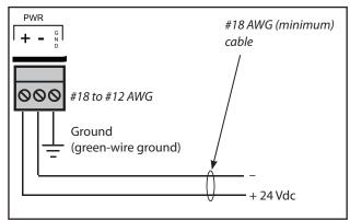
Note: The common connection from the 24Vdc power supply should **not** be connected to green-wire ground unless specified by local electrical codes.
