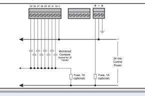
Note: 18 AWG (Belden 8760) shielded twisted pair cable is recommended for all input and output connections.
